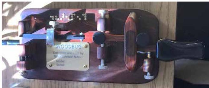
This bug was hand built by NA6O Gary Johnson. The tensions are magnetic and the dit contact is a magnetic switch.
